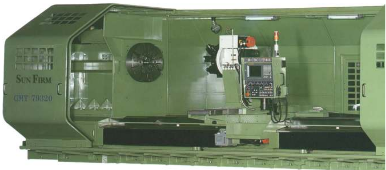
CMT 79320 with C Axis & D.R.O. for X, Z Axis
